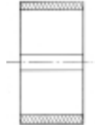
Style B Flush both ends. Standard design on wheels under 6" dia.
